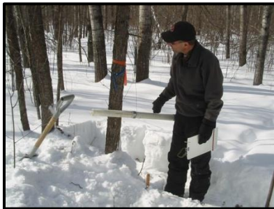
Establish base weight of empty sampling tube
