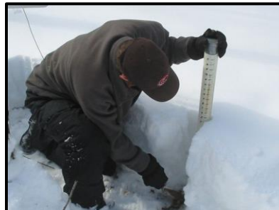
Obtaining snow depth and core sample
